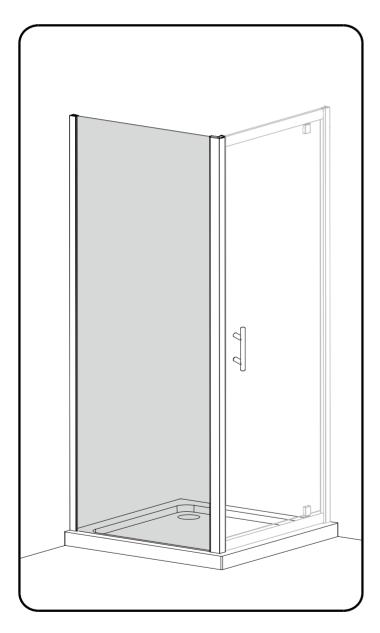
Note: Instruction shows fitting of a Side panel with a Pivot door as an example only. This Side panel can fit with the Sliding door, Bi-fold door, and Hinge door etc.
